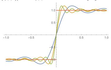
The blue curve corresponds to a Fourier series with 10 terms, the yellow one with 20 and the green one with 30 terms. Observe that at x=0 (the point where f is discontinuous) all the truncated Fourier series pass through the origin —this is consistent with the theory about convergence discussed previously, Theorem 1.2.
