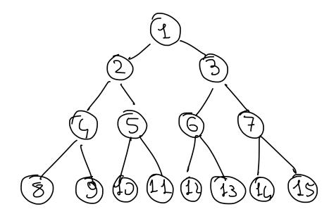
The network is onnected with N=15 modes and L=14=N-1 links therefore it is a tree
