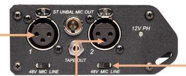
Each input onto the mixer has a MIC/LINE/48V switch. If you are attaching a mic – select MIC. If the mic needs phantom power – select 48V. A radio mic does not need phantom power. A boom mic usually does, but check.
