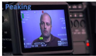
WFM gives access to a number of video scopes. The 2<sup>nd</sup> option is the **edge monitor** which shows the distribution of sharpness across the image. As sharpness increases a pattern of peaks appear across the bottom of the LCD.
