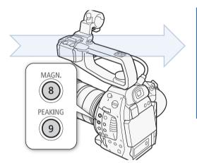
**Magnification** enlarges the image so more detail can be seen and focusing is easier.
