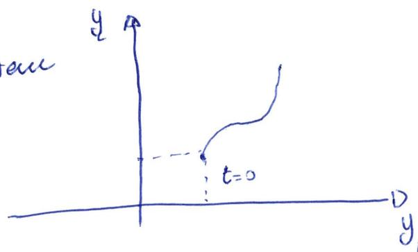
A region of the two dimensional space  $\mathbb{R}^2$  described by the coordinates  $(y_1, y_2)$  where the functions  $f_1(y_1, y_2)$  and  $f_2(y_1, y_2)$  are well defined is called the PHASE SPACE of the system.
