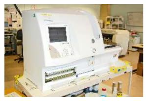
In the laboratory the full blood count is determined by one of these machines. The sample is shaken to ensure even distribution of cells and bottles are loaded in. It can process 120 samples per hour.
