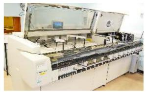
The Abbott Architest integrated general chemistry & immunoassay analyser will process 1200 clinical chemistry and 200 immunoassays per hour. Only one serum specimen is needed for both.
