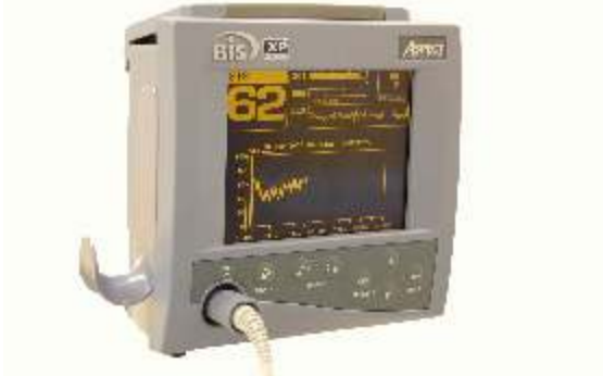
Bispectral index cerebral function monitor. It monitors the depth of anaesthesia by recording electrical activity (Electroencephalography or EEG)
