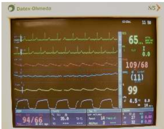
The video monitor during a major case. It shows ECG, pulse rate, blood pressure, O 2 saturation, expired CO 2 , central venous pressure, direct arterial pressure & temperature
