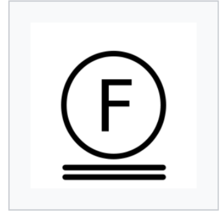
Very gentle cleaning with hydrocarbon solvents
