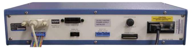
**Digital signal input port** - an 8-bit digital input port is provided to reach switch positions, etc.
