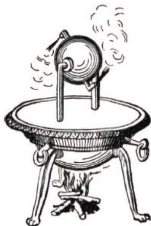
Hero of Alexandria, device to convert heat into mechanical energy
