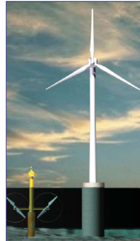
Greater energy intensity in tidal currents allows a smaller device to generate the same power. This image compares 1 MW wind and tidal turbines.
