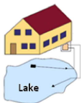
Fig. 5. Open loop system using surface water (redesign) [56].
