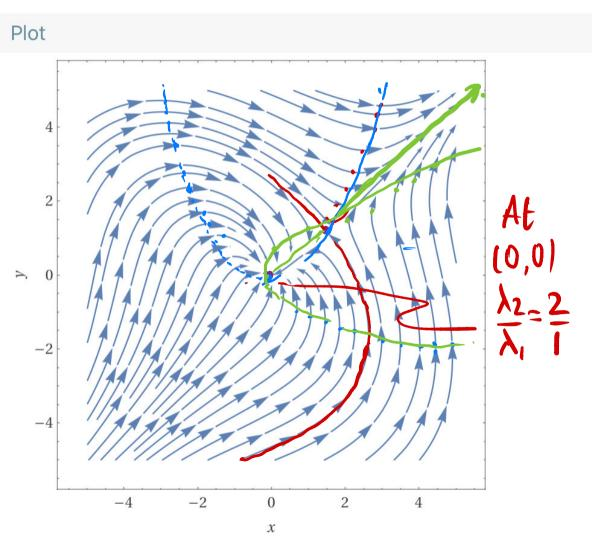
Streamplot $\{-x+y^2,-2y+x^2\}$  x from-5 to +5, y from -5 to 5
