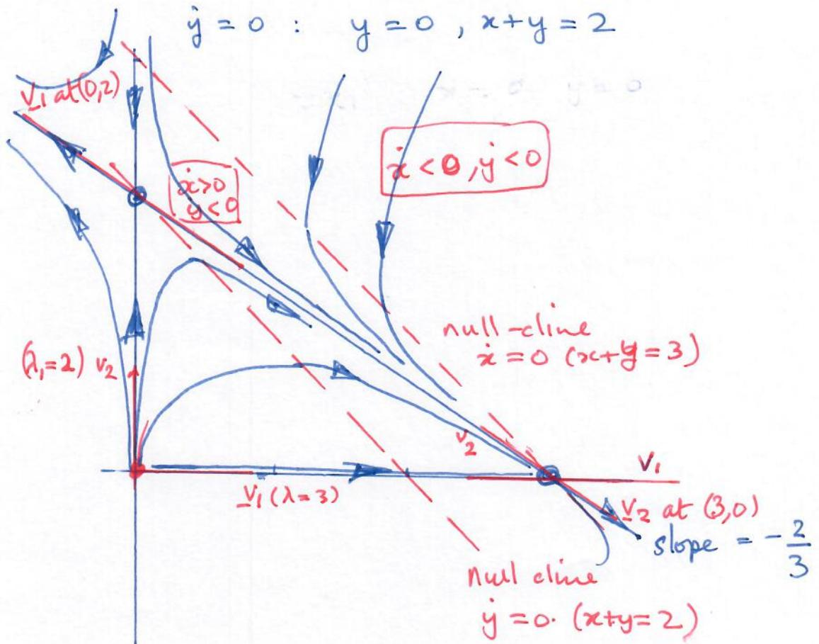
Fixed points  $x_1^*, x=0, y=0$  $x_2^*, x=0, y=2$  $x_3^*, x=3, y=0$
