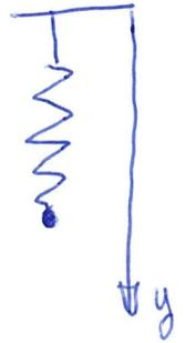
$$\text{ODE: } m\ddot{y} = mg - k(y-l) - \gamma\dot{y}$$
