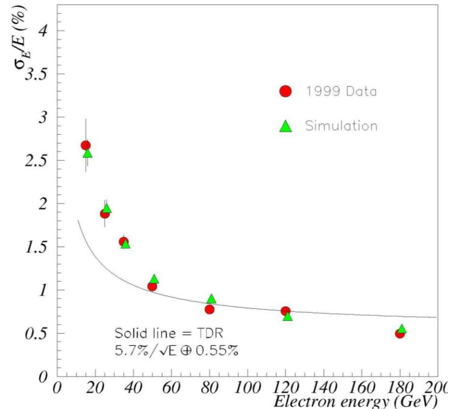
Energy resolution degraded by Pb absorber
