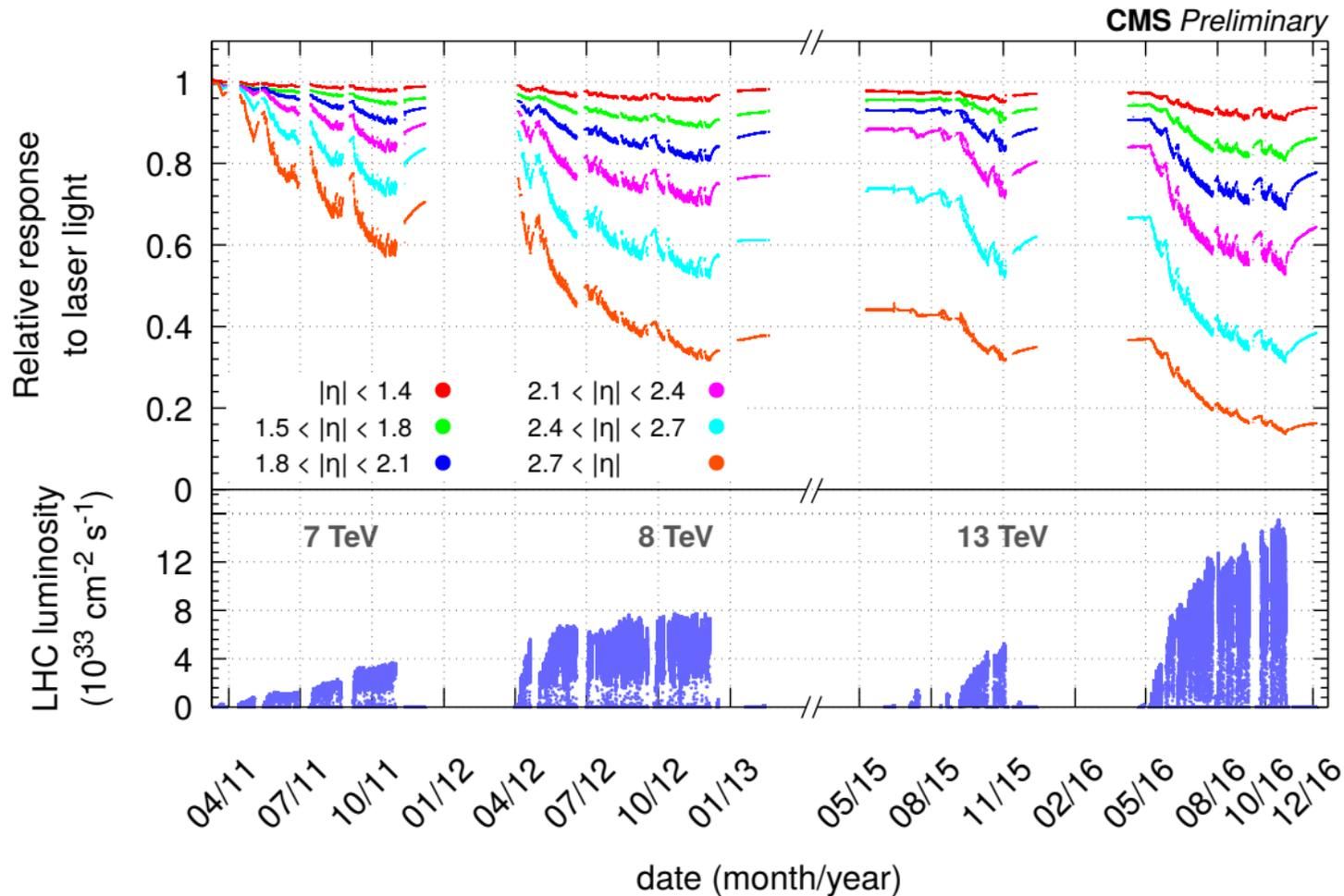
Relative response to laser light (440 nm) measured by the laser monitoring system, averaged over all crystals in bins of pseudorapidity, for the 2011 through 2016 data taking periods
