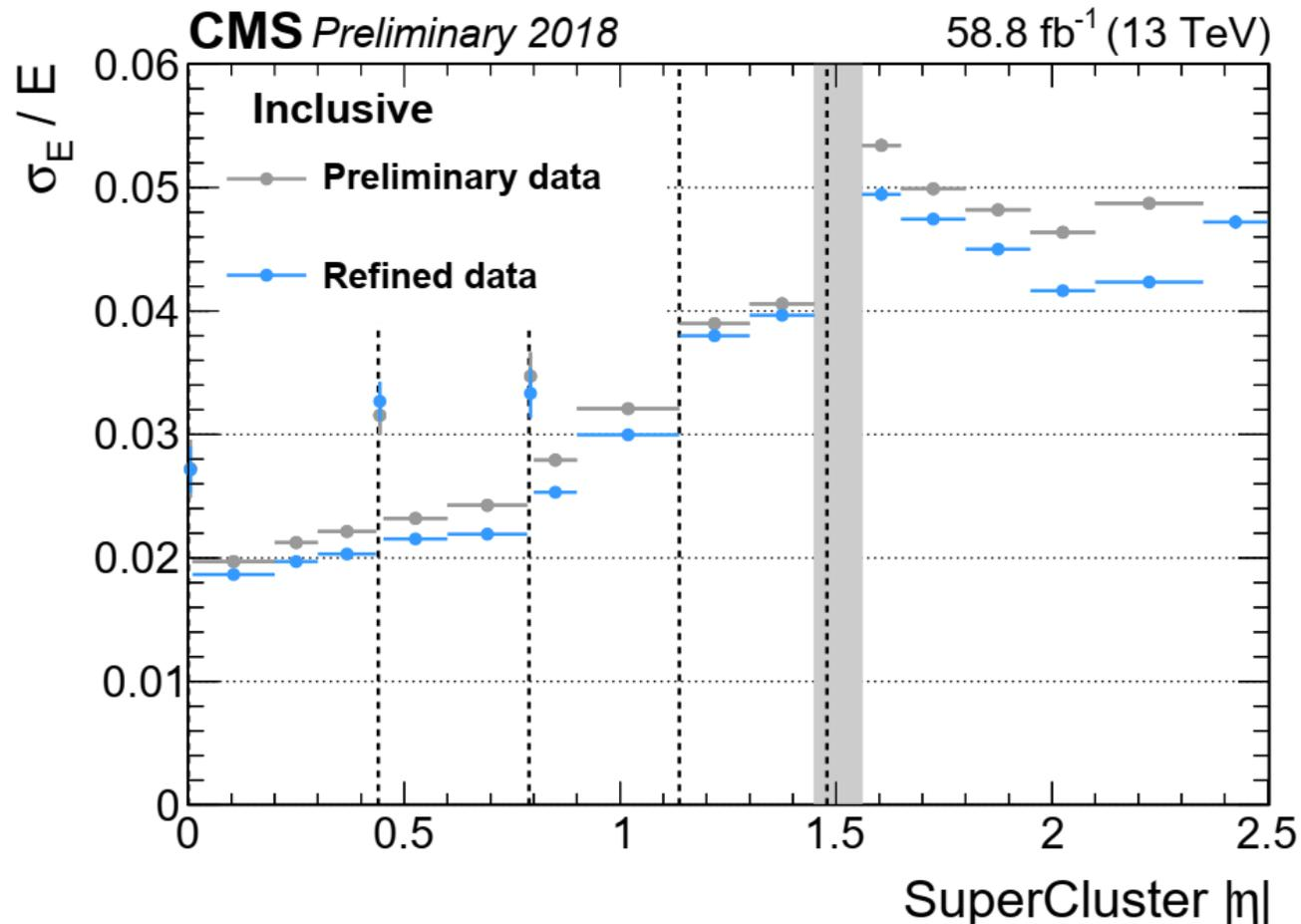
The plot shows the  $Z \rightarrow e^+e^-$  energy resolution. The region with the vertical grey bar is the physical join between the barrel and the endcap region.
