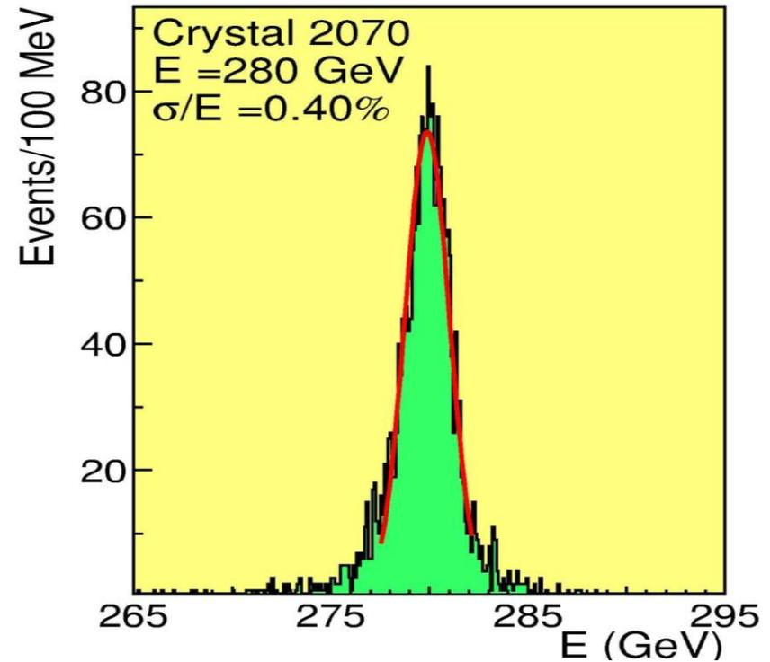
Barrel specifications:  $\frac{\sigma_E}{E} = \frac{2.7\%}{\sqrt{E}} \oplus \frac{155 \text{ MeV}}{E} \oplus 0.55\%$
