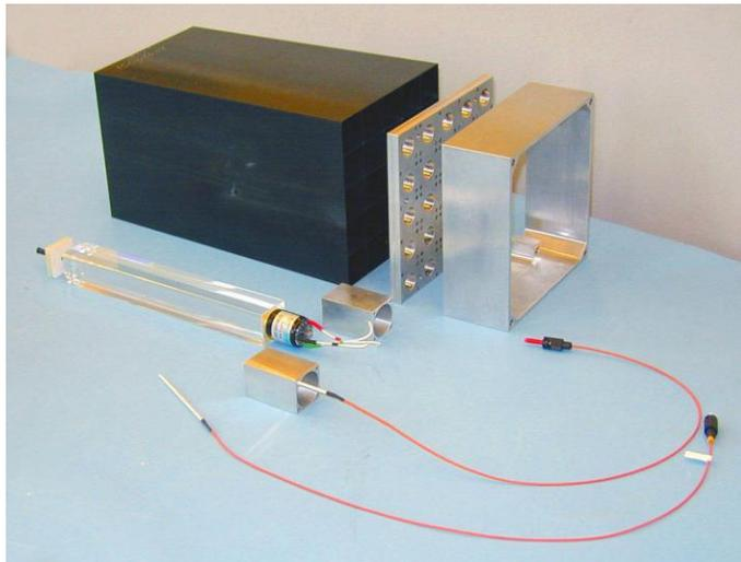
**'Supercrystal'**: carbon-fibre alveola containing 5x5 tapered crystals + VPTs + HV filter
