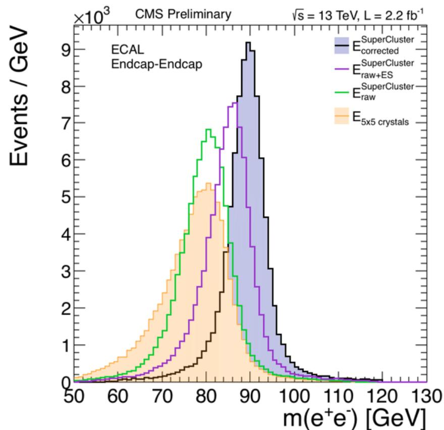
The two plots show the improvements to the  $Z \rightarrow e^+e^-$  energy scale and resolution from the incorporation of more sophisticated clustering and cluster correction algorithms (energy sum over the seed 5x5 crystal matrix, bremsstrahlung recovery using supercluster, inclusion of preshower (ES) energy, energy correction using a multivariate algorithm).
