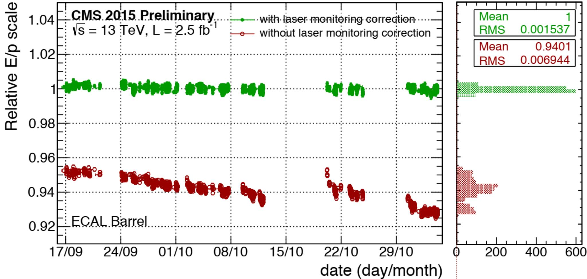
Correcting for the effects of radiation damage using the laser monitoring system. Barrel calorimeter shown here. In 2015 the average signal loss ~6% for ECAL Barrel, rms stability *after corrections* was 0.14%
