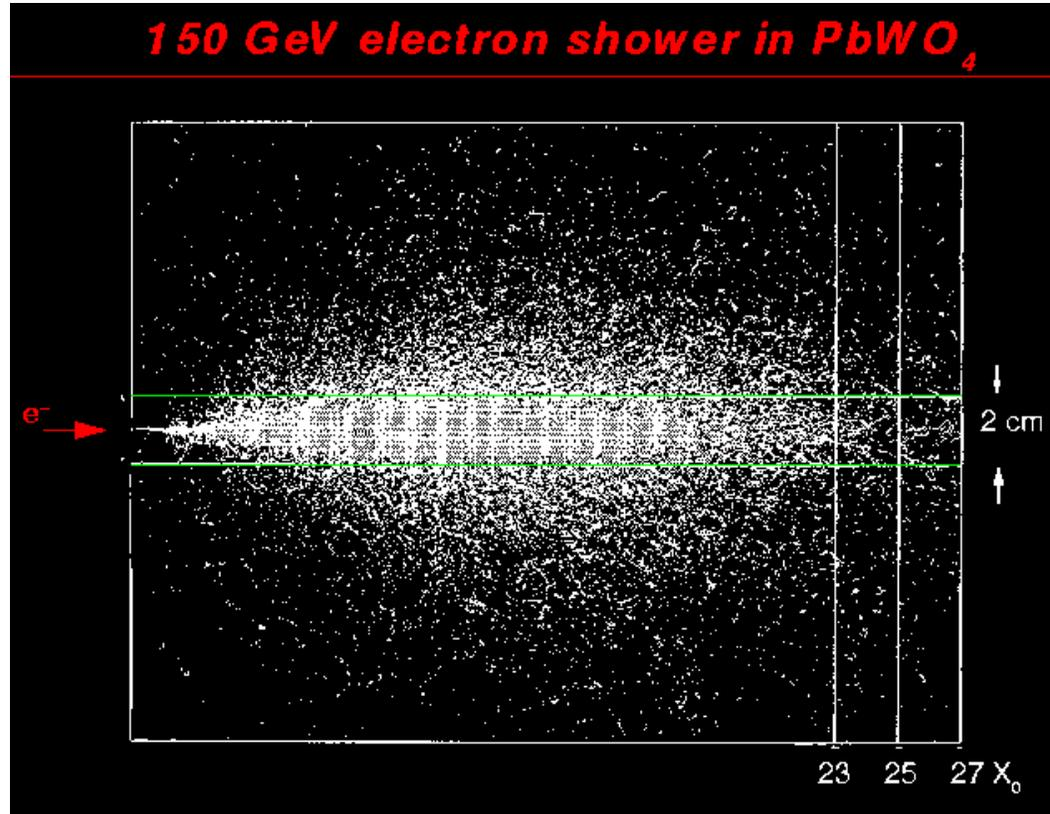
CMS Homogeneous ECAL scintillator simulation. The green lines show the approximate location of a single crystal.
