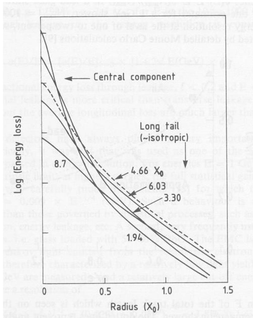
Calorimeter cells are typically one Moliere radius in size. Some lateral shower sharing between cells improves the position resolution.
